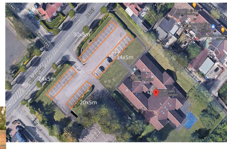
This car park is closed during the night time. The proposal is to install 42 x 7 kW charging bollards and make them accessible to the nearby residents (up to 10mins walking distance) who do not have off street parking facility. Battery will allow for a smaller grid connection.
