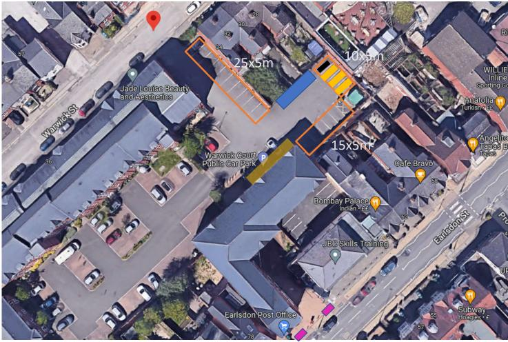
The proposal is to install 15 x 7 kW charging bollards and make them accessible to the nearby residents (up to 10mins walking distance) who do not have off street parking facility. Battery will allow for a smaller grid connection.
